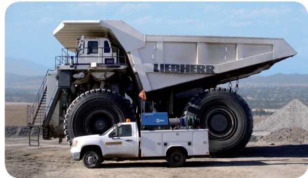
The Liebherr T 282 C is the most powerful mining truck in the world: It can carry up to 363 metric tons at a top speed of 40 mph
