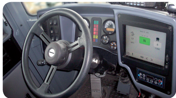
The Kontron heavy-duty industrial PC ThinkIO displays important information on payload, faults, temperatures etc on a graphic display in the driver cabin.
