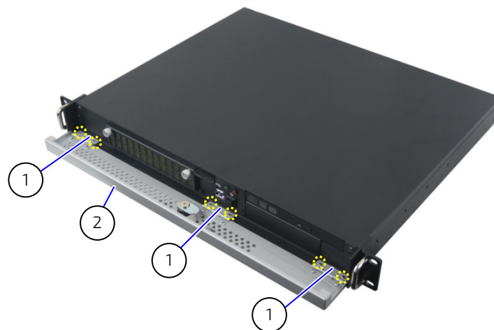
Figure 26: Removing the front access panel
