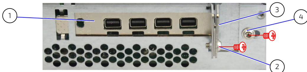
Figure 22: Rear side with slide bracket closed (for fixing the expansion card/slot bracket)
