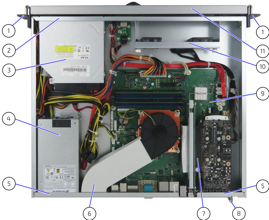
Figure 18: Example of KISS 1U Short V3 configuration with mainboard and low-profile expansion card
